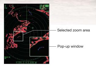
With the optional ARP board ARP-11, up to 10 targets can be acquired and tracked on the radar screen. Additionally, up to 100 AIS targets can be presented with appropriate AIS data input.
